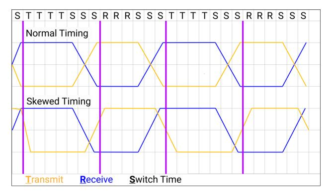
Figure 2: Ideal timing of TDD switches exhibit extreme precision, with handoffs occurring uniformly within the delay frames between transmit (yellow) and receive (blue) operations. Skewed timing caused by propagation delay, for example, can lead to switching overlap and leading data errors, among other challenges, which decreases the integrity of TDD transmissions.
