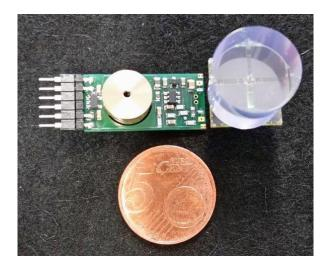
Bias generator / preamplifier for SiPms CsI(TI)
