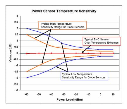
Figure 1 - Temperature Sensitivity of Model 12100 versus Typical Diode Sensors
