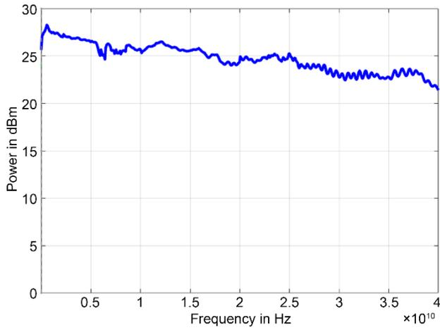
Figure 6: Max Output Power 0.01 to 40 GHz
