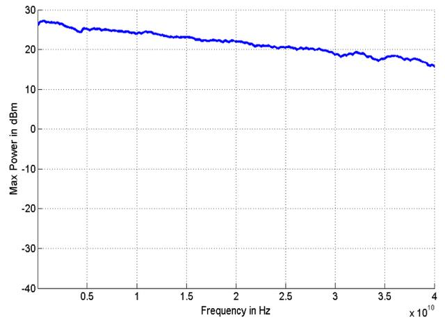
Figure 7: Max Output Power 0.01 to 40 GHz
