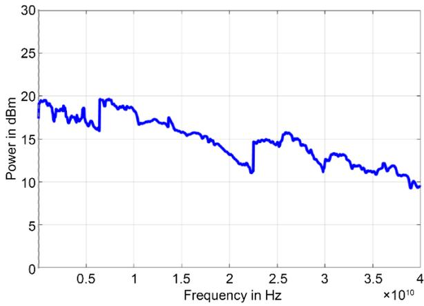
Figure 8: Max Output Power 0.01 to 40 GHz
