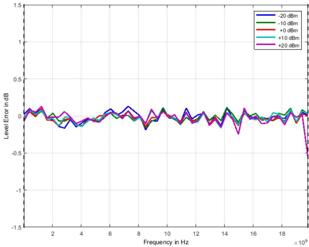
Figure 11: Typical Output Power Linearity (Model 865B-20)
