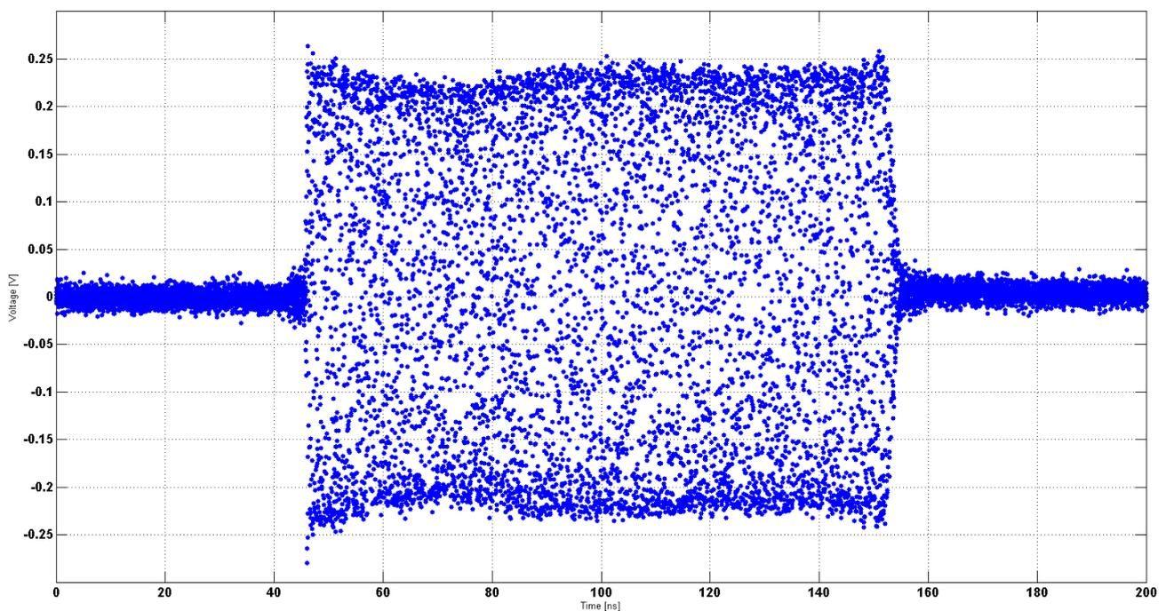
Figure 13: Model 865B-40 option NP or NEC Pulse Modulation 30 ns - 40 GHz Carrier Frequency
