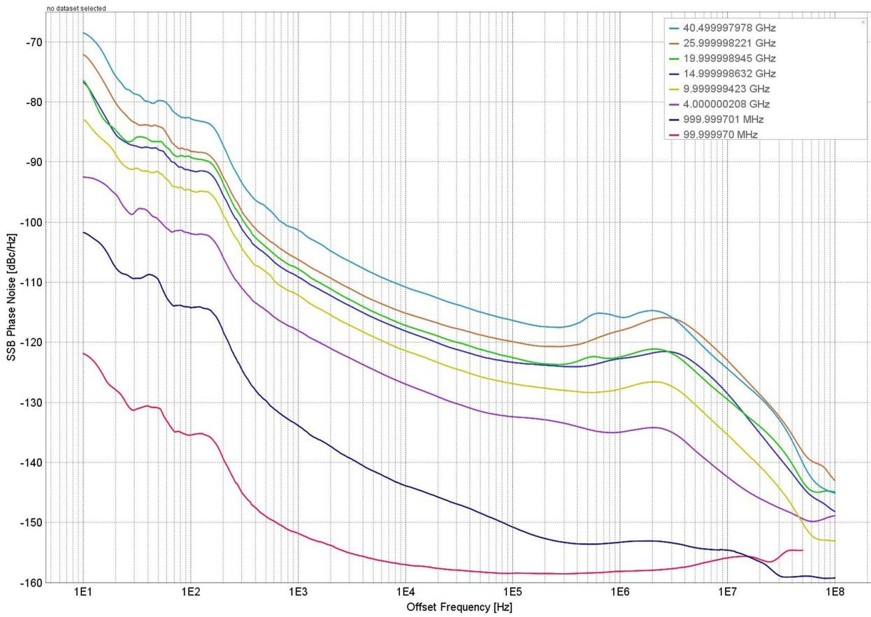
Figure 2: SSB Phase Noise Performance, without option LN
