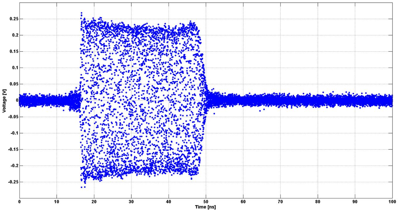
Figure 14: Model 865B-40 option FS Pulse Modulation 20 ns - 40 GHz Carrier Frequency
