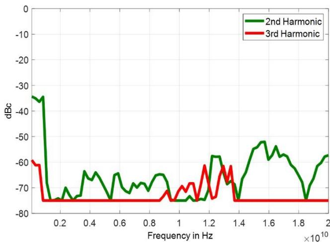
Figure 4: Harmonics (2nd, 3rd at P=5 dBm, 865B-20)
