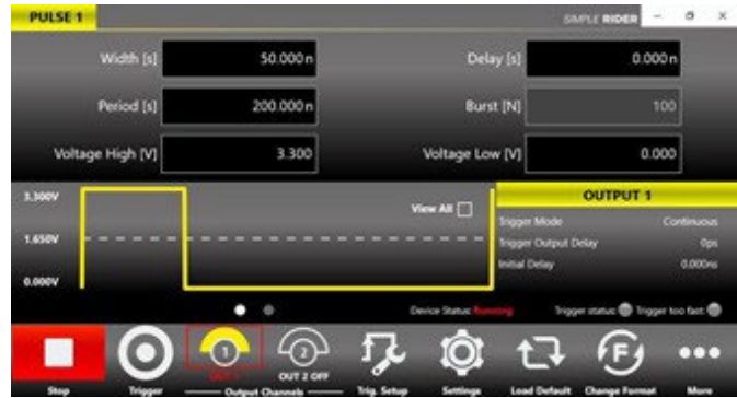
Figure 1: Model 765 setup to program or erase a single cell: pulse characteristics: 50 ns @ 3.3V
