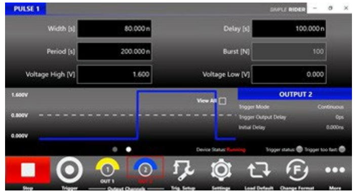
Figure 5: Model 765 setup for a “large” pulse 80ns @ 1.6 V (Set Pulse)
