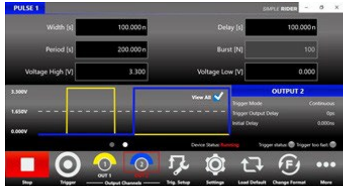
Figure 2: Model 765 setup to program or erase an array of cells: pulse characteristics: 100 ns @ 3.3V
