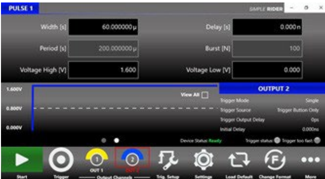
Figure 11: Screen UI “slow pulse” baseline -1V, max 2V2 (amplitude 3,2V) duration 60 us single mode
