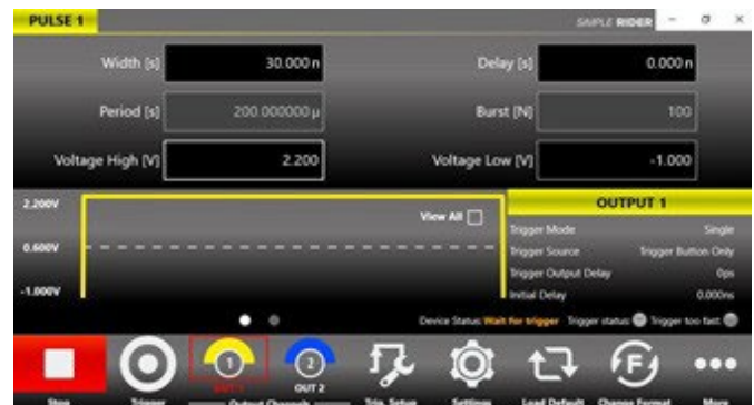
Figure 9: Screen UI "short pulse" baseline -1V, max 2V2 (amplitude 3.2V) duration 30 ns single mode
