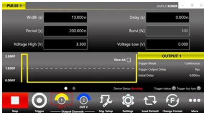
Figure 4: Model 765 setup for a narrow pulse 10ns @ 3.3V (Reset Pulse)
