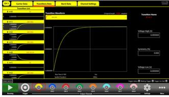
The software architecture provides the possibility to easily generate the patterns in different generation modalities and also gives the opportunity to modulate the patterns with internal or external signals with the purpose to generate also different effects of noise (jitter, ripple, ...).
