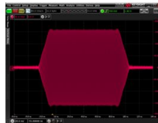
Figure 11. 100 ns pulse with 16 ns rise/fall times.
