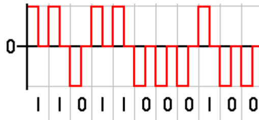
Figure 3: Baseband Return Zero code.
