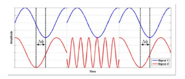
With 2 phase coherent signals at frequency (F1) and relative phase  $(\omega)$ , signal 2 undergoes frequency switching (F1, F2, F1). Following the sequence, the 2 signals once again have the same relative phase  $(\omega)$ .
