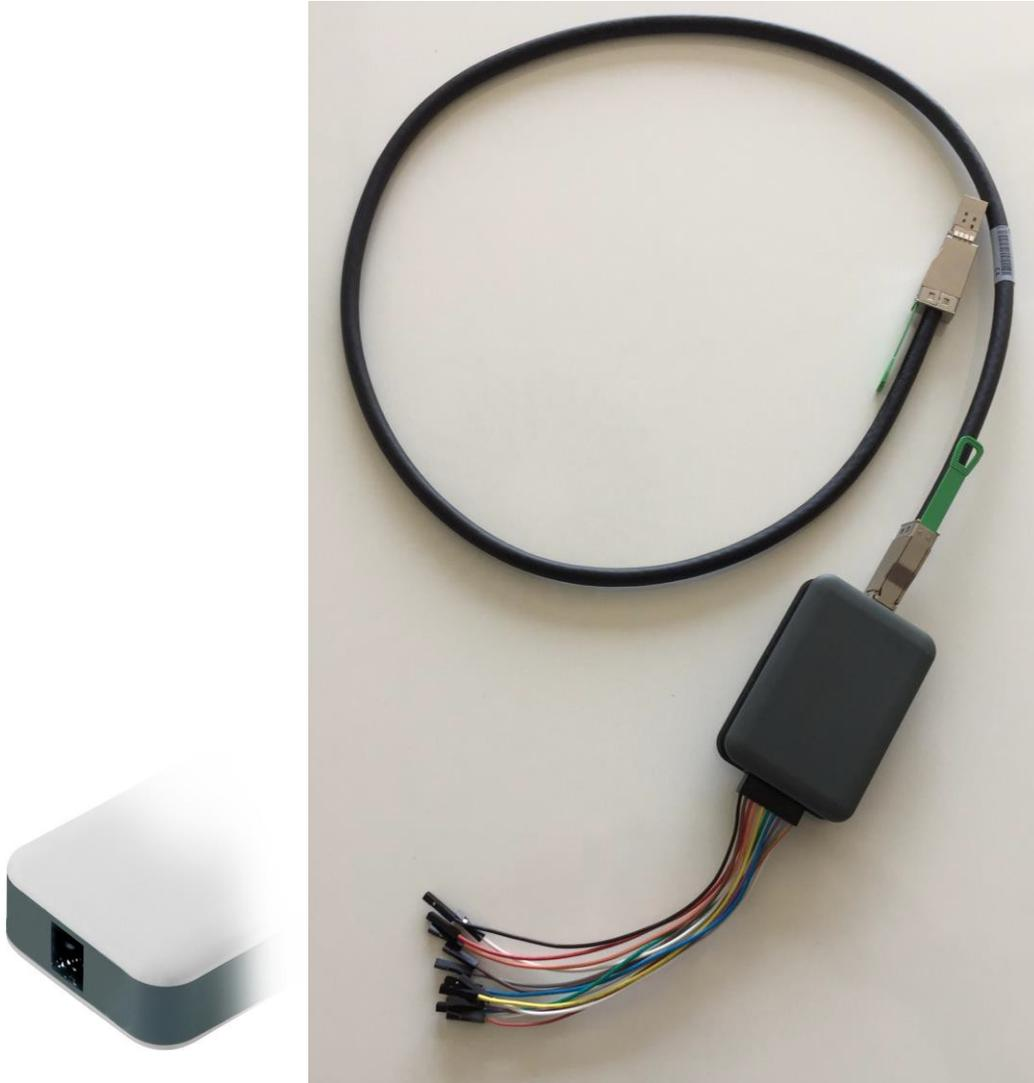
An 8-bit LVDS to LVTTL converter has been developed and can be used to convert LVDS differential signals to LVTTL single ended signals with a software programmable voltage level from 0.8V to 3.8V.
