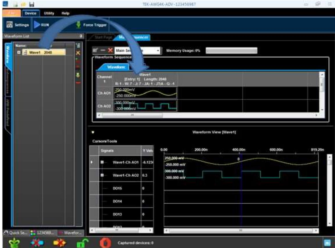
15. Now, press the Run/Stop button on the AWG4K toolbar.
