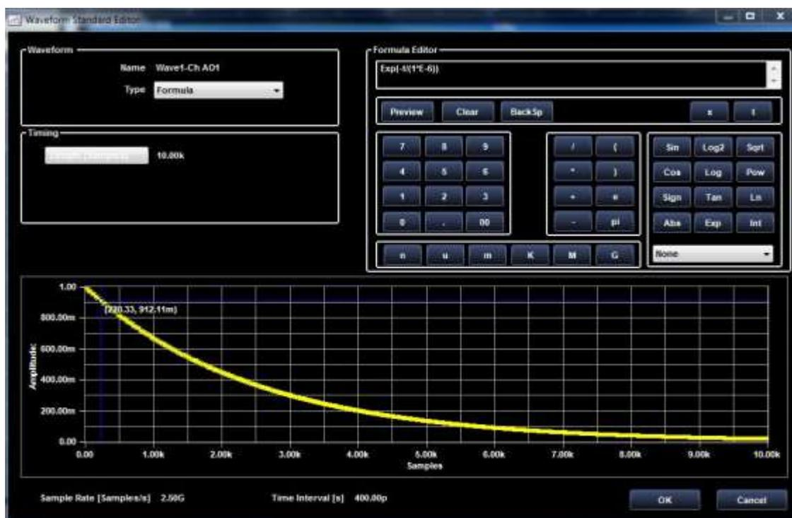
A decaying exponential waveform. The actual formula used here is  $\text{Exp}(-t/(1*E-6))$ .
