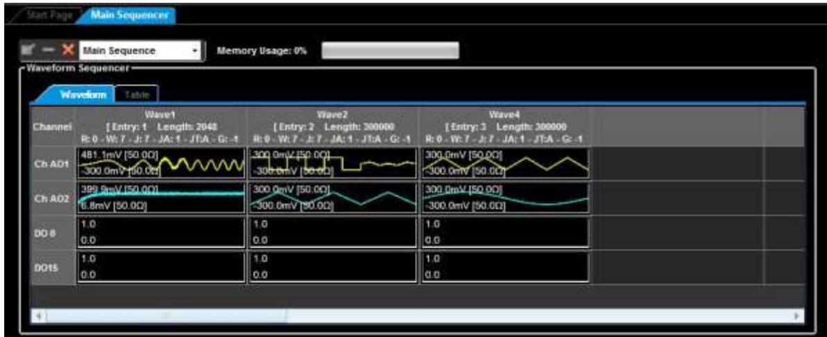
**Single Sequencer** projects have one sequencer called Main Sequencer that controls all analog/digital channels waveform generation.
