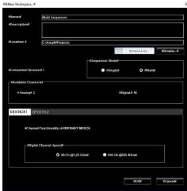
5. Select the **Digital Channel Speed**: in ARB mode it is possible to operate with all of the 32 channels with a maximum update rate of 625MSps or with half channels (16) at 1.25Gbps.
