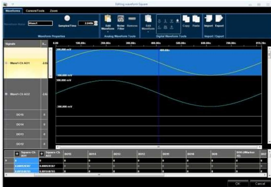
5. The Waveform Standard Editor is shown. Choose a sine waveform with the following specs:
