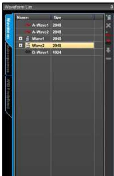
The Waveforms TAB has a toolbar on the aside allowing you to Add, Delete or Copy the waveforms.
