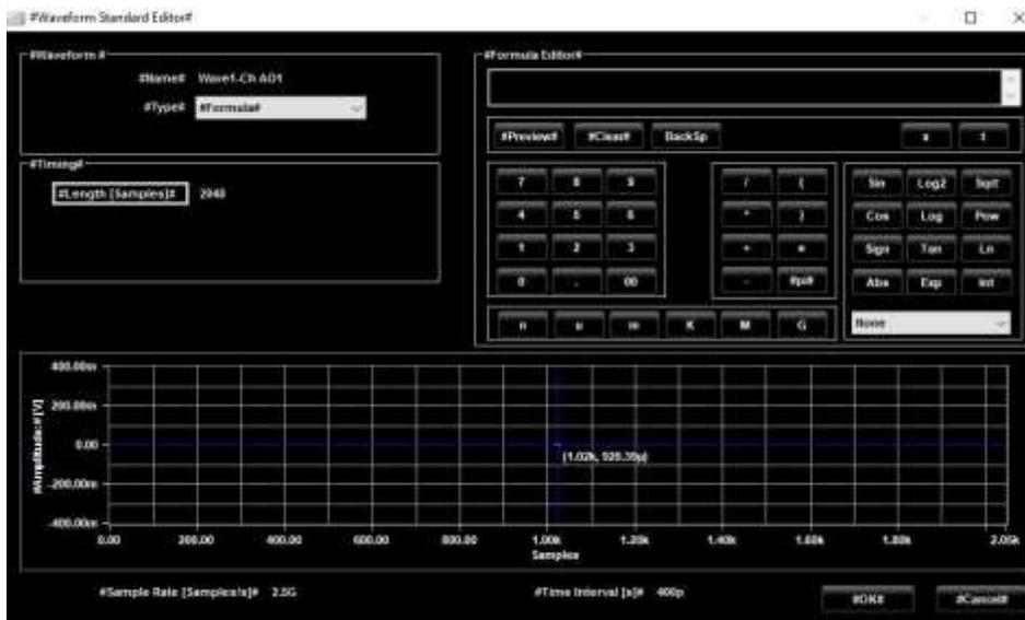
On the Type drop-down list select *Formula*. The Formula Editor is then shown on the right. The editor helps building your waveform analytically using equations. Your equation can be based on time(*t*) or samples(*x*).
