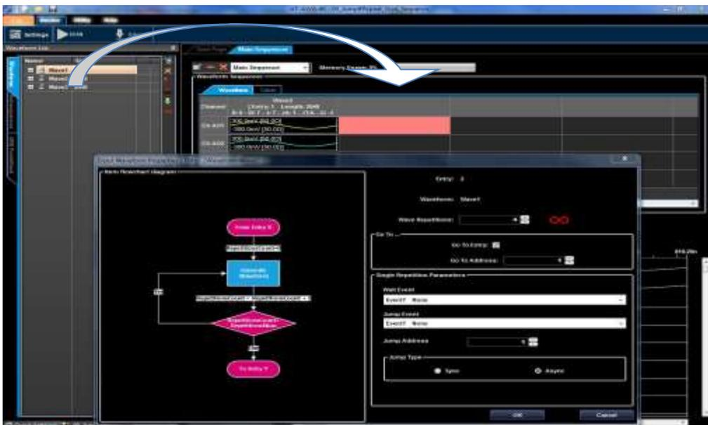
On the *Input Waveform Properties* window select 4 repetitions, mark the Go To Address checkbox and type 1 as Go To Address value. Press OK to confirm.
