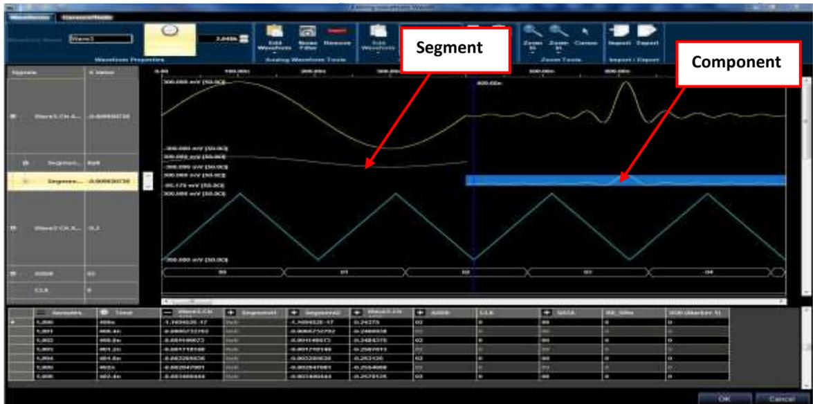
The waveform in the picture above is the composition of two segments. Each segment is made of one component.
