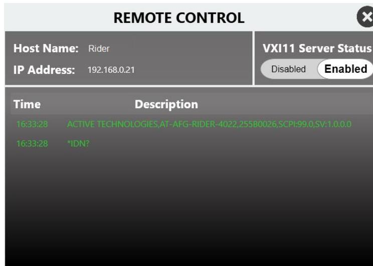
In the top of the page you can read the Host Name and the IP Address of the instrument. The slider allows to enable or disable the SCPI server, by default it is enabled.
