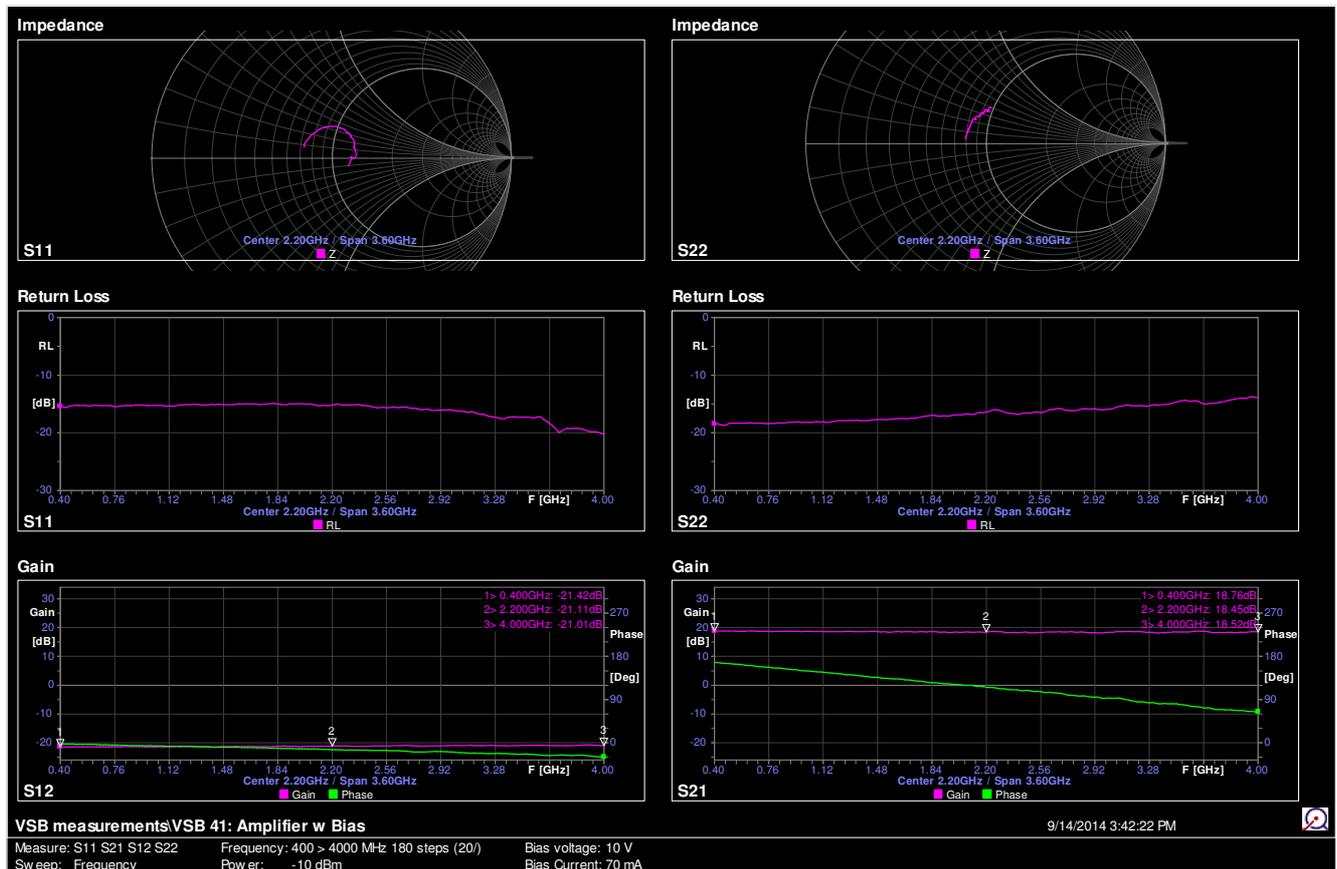
The amplifier has a steady gain of 18.5dB which varies by only 0.25 dB up to 4 GHz. The reverse gain is about -21dB, which shows that the amplifier is stable. The return loss is also around a nice 15dB over the frequency range.
