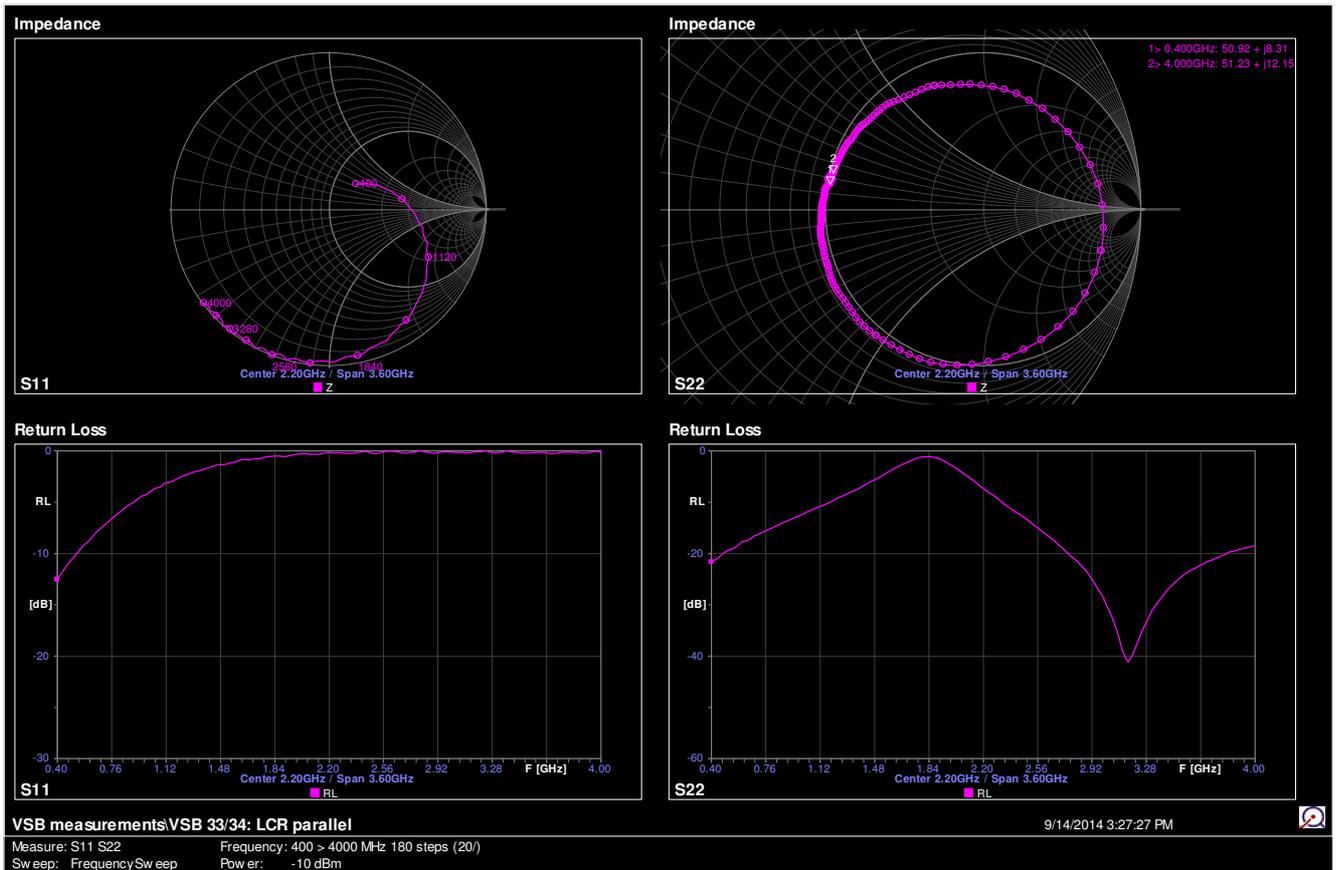
Notice that the frequency indications in the Smith chart give a much better insight in the circuit's behaviour than the bare lines that other VNAs show. These markers are a unique feature of the VNA0440e software. In the right Smith chart the measure point markers are turned on.
