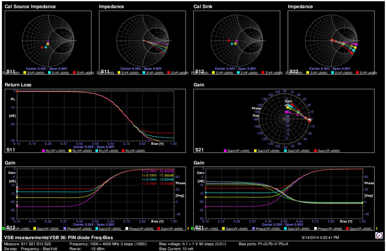
We can see how the impedance and attenuation develop over bias voltage, at each of the frequencies.
