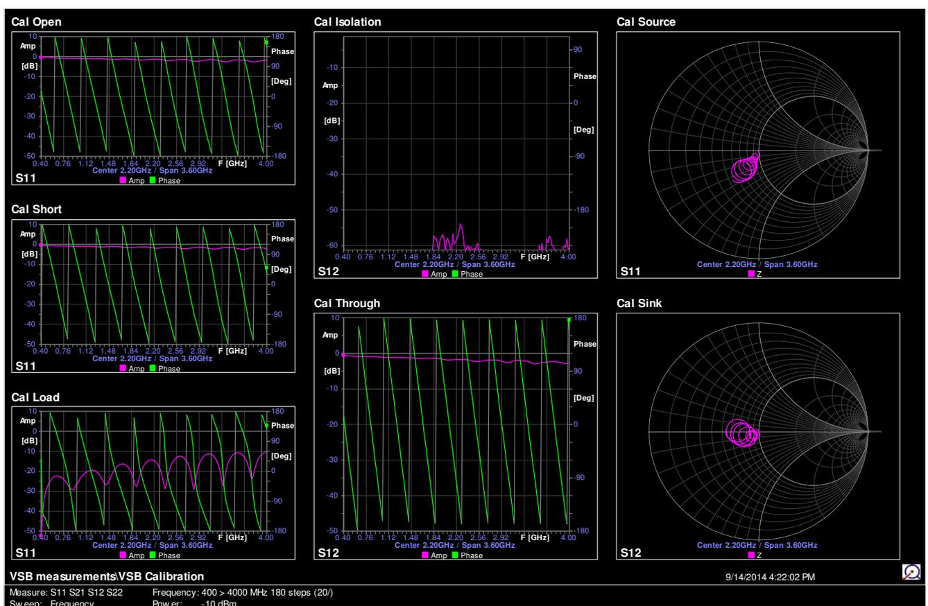
From the Open-Short-Load calibration (the three graphs on the left), the VNA0440e calculates the impedance at the reference plane of the calibration. This is the Source impedance with which the circuit under test is excited.
