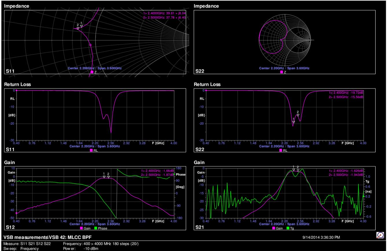
This filter has a 0.3dB variation in Insertion Loss and a good Return Loss in the Wifi – Bluetooth – Zigbee band from 2.4 GHz to 2.5 GHz. The fairly high Group Delay (Gain S21, green trace) may distort signals and cause symbol errors in an application.
