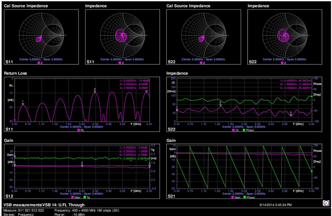
The total impedance and gain varies quite a bit over the frequency range and the return loss is quite low on some frequencies. This should be taken into account when applying these cables in an RF application.
