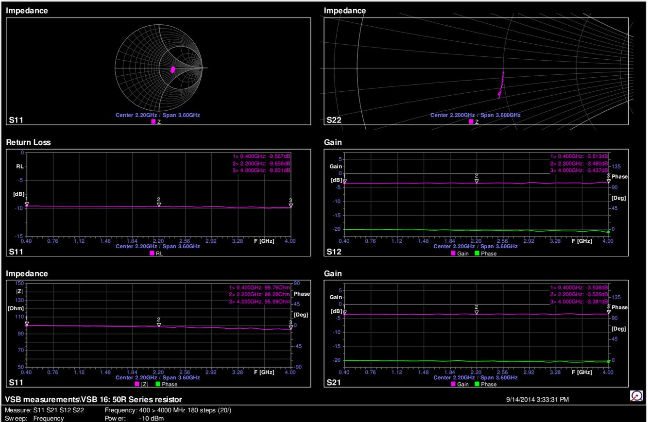
In series with the system impedance of 50 Ohm we measure (nearly) 100 Ohm in total. The circuit has about 3.5dB attenuation.
