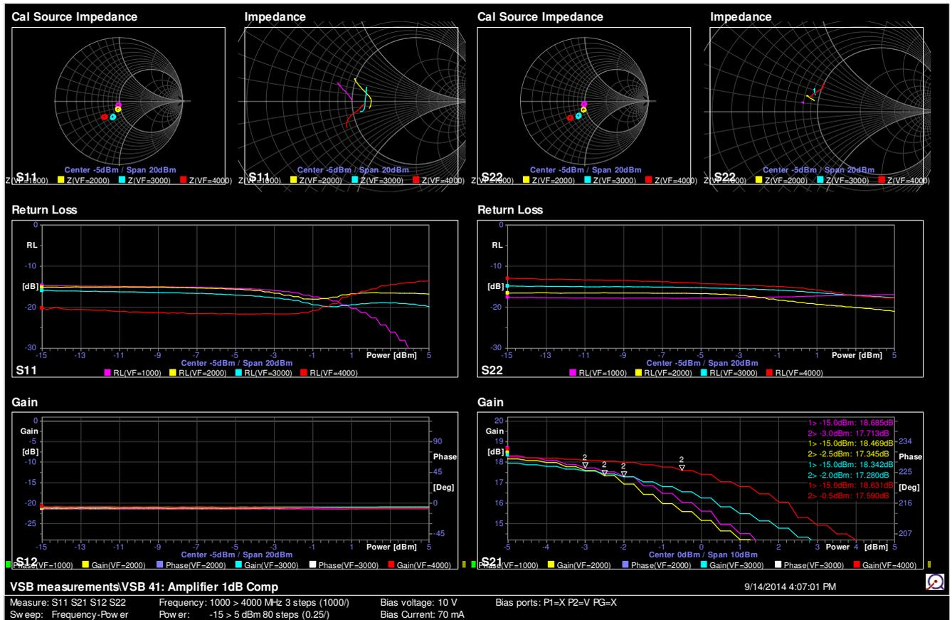
We determine the level at which the gain decreases by 1dB by setting a marker at the low frequency gain (outside the zoomed graph) and finding the point at which this gain is 1dB lower. The compression point is measured at 1, 2, 3 and 4 GHz.
