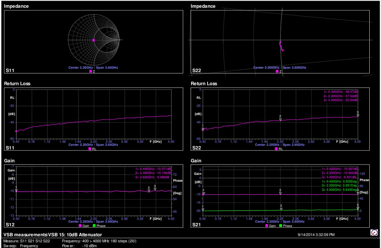
A simple resistor network has very accurate attenuation and matching over the whole band, with only 0.2 dB variation in attenuation.
