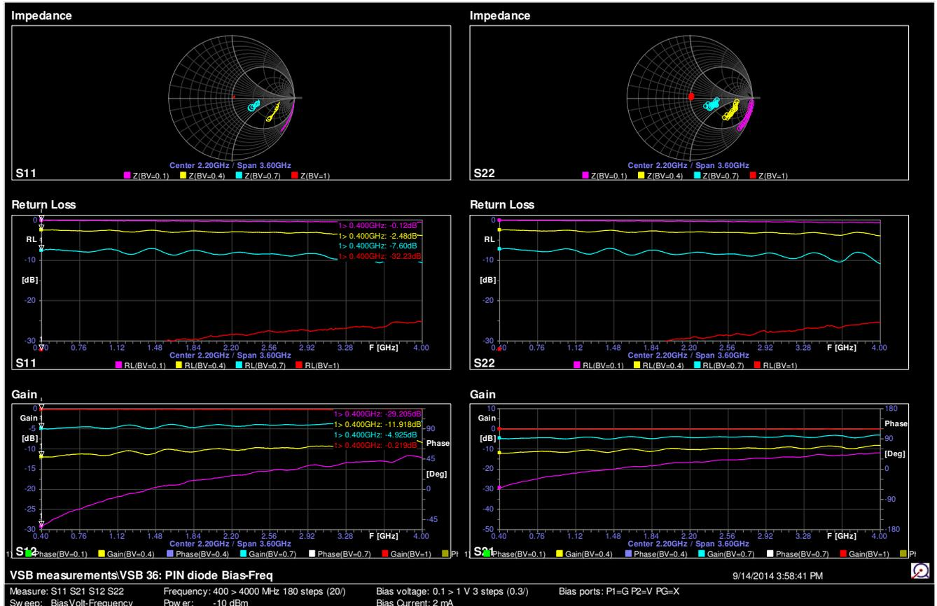
At the highest voltage (red traces) the PIN is turned ON and it is a good bypass, connecting the 50 Ohm measuring source directly to the 50 Ohm termination impedance. When the voltage gets lower (towards the purple traces) the PIN becomes a series resistor. The attenuation is highest at the lower frequencies.
