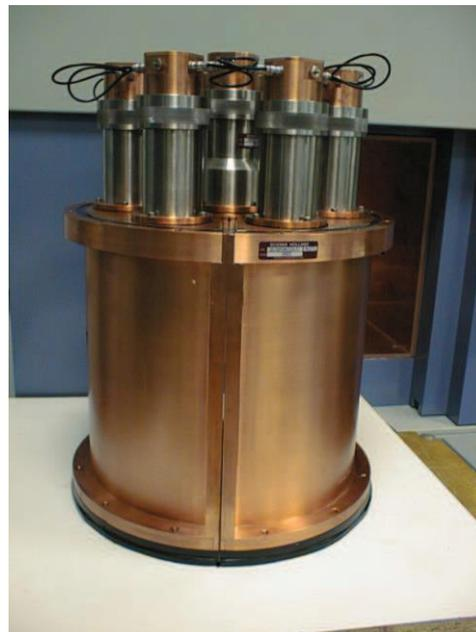
Examples of NaI(Tl) Anti-Compton shields for low level detection
