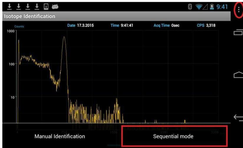
Figure 4.26. Starting Sequential mode
