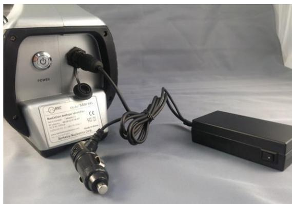
Figure 3.8. Detector unit (rear view) and vehicle adapter/charger
