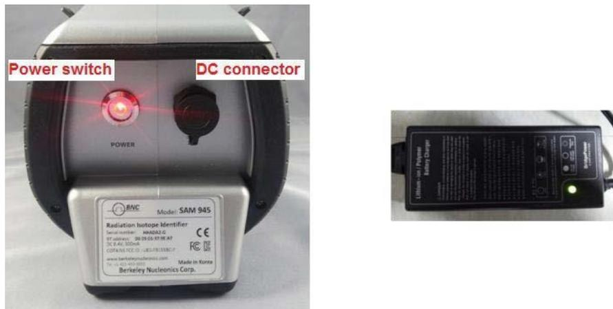
Figure 3.7. Detector unit (rear view) and AC adapter/charger
