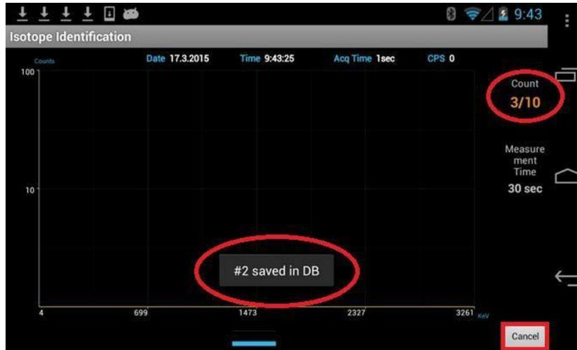
Figure 4.28. Sequential mode example showing pause between event captures
