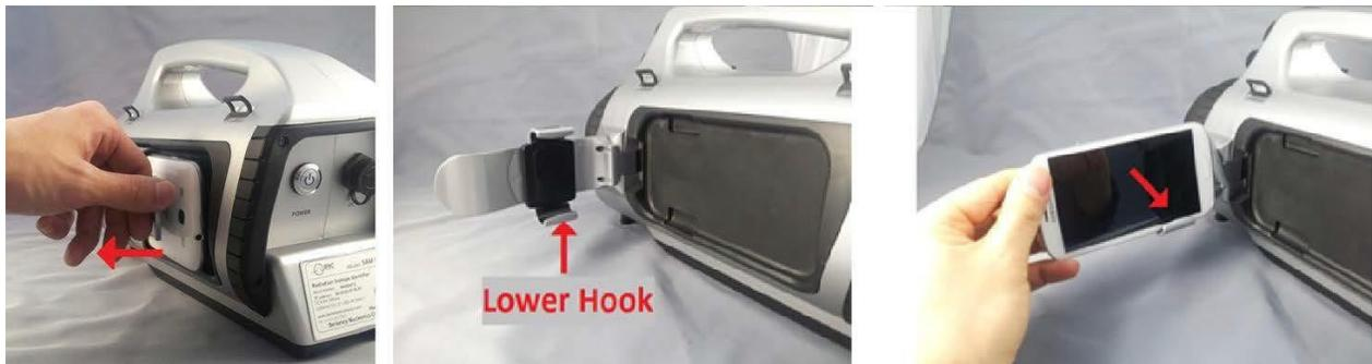
Figure 3.3. Attaching the smartphone to the detector
