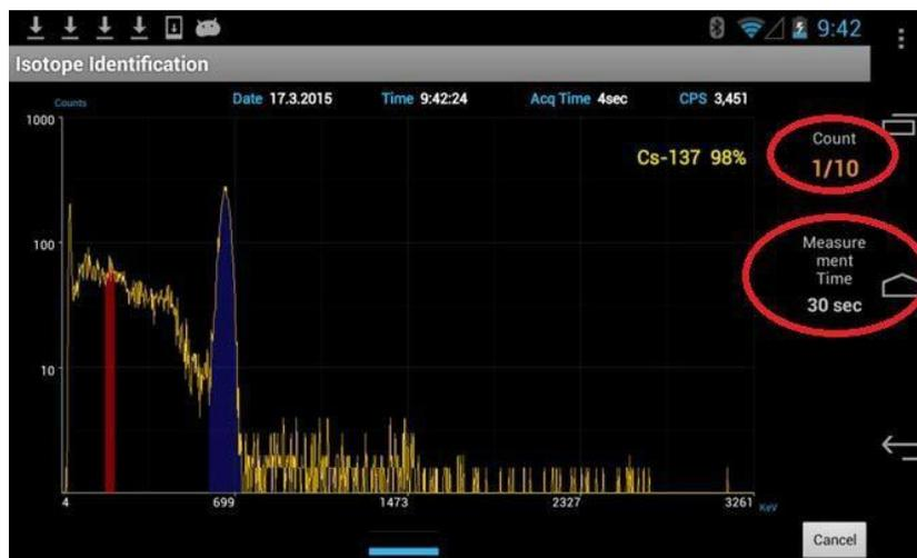
Figure 4.27. Sequential mode event capture example
