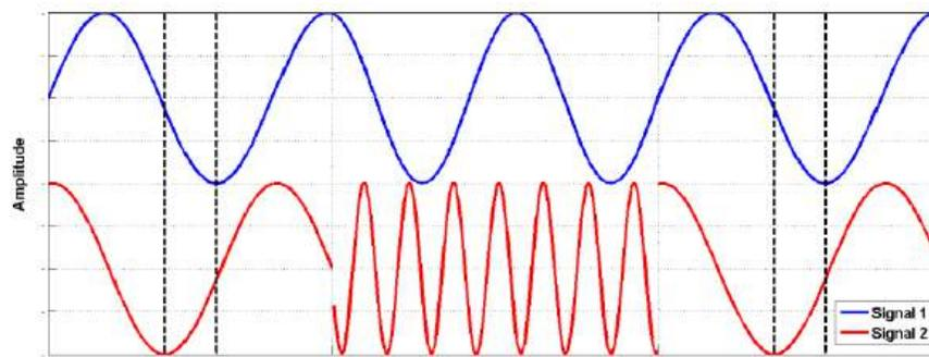
The relative phase between channels 1 and 2 (signal 1 and 2) remains the same after channel 2 temporarily switched to a different frequency. The frequency switching itself is phase discontinuous because the original phase is restored.
