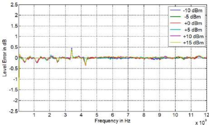
**Figure 5: Power Level Accuracy 875-12**
