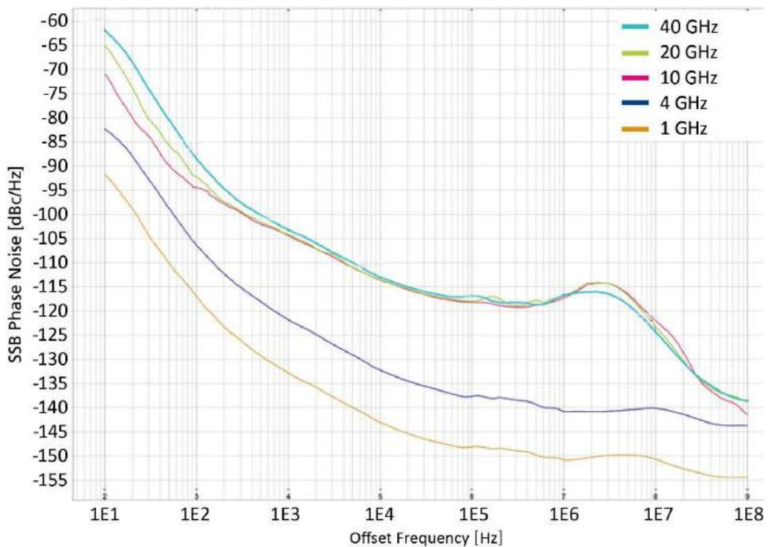
Figure 11: SSB Phase Noise Performance, 875-XX, low frequency CW without option LN, Pout = +10 dBm
