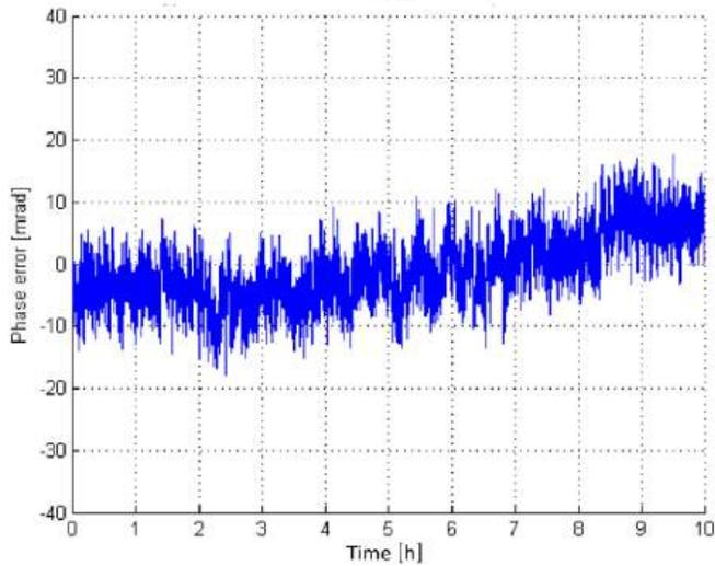
Figure 18: Phase coherence performance at 15 GHz
