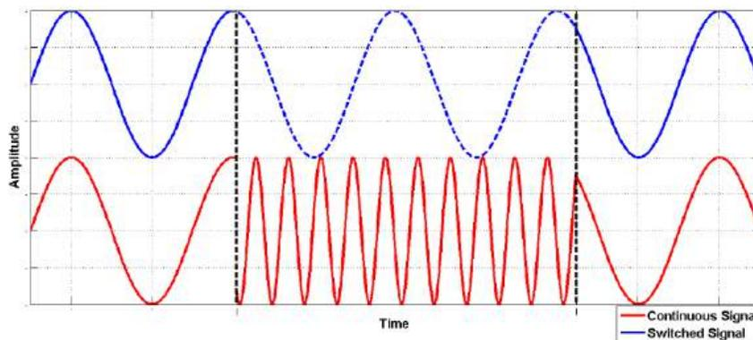
The signal returns to the same absolute phase when returning to the previous frequency and amplitude setting.
