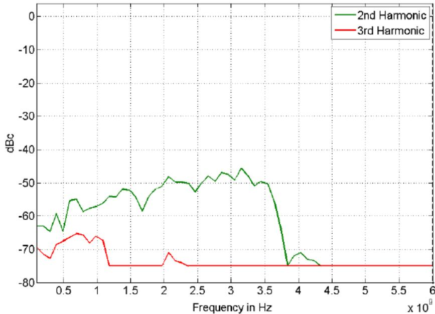
Figure 14: 875-20 – Harmonic Performance at Pout = 0 dBm
