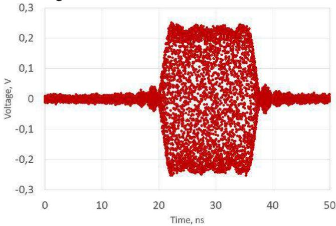
**Figure 24: Pulse modulation 16 ns at 40 GHz**
