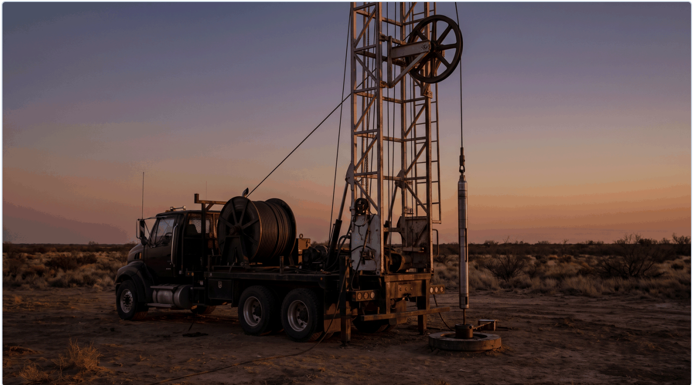
■ ILLUSTRATION Figure 2. A wireline logging unit at a well site, with the tool string at the wellhead; no real site is depicted.
