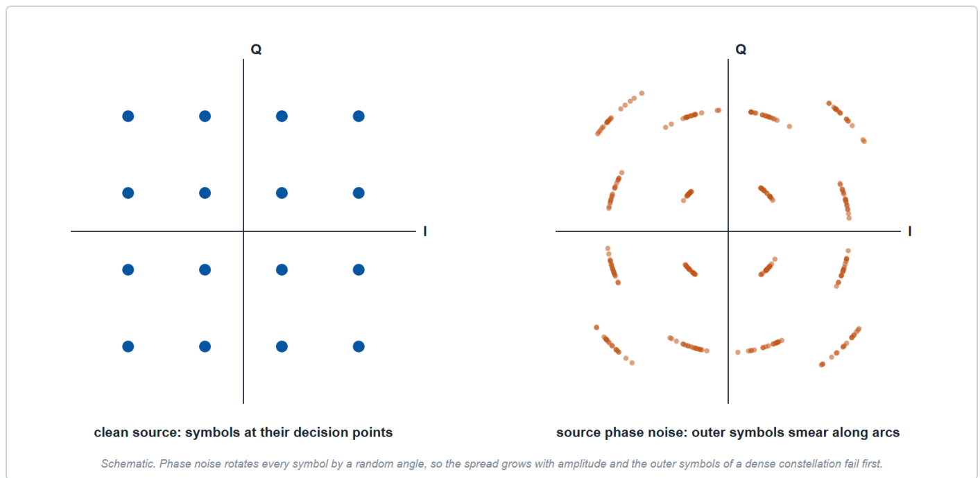
■ SCHEMATIC Figure 2. A clean 16-QAM constellation and the same constellation with source phase noise; the random rotation spreads the outer symbols along arcs first.
