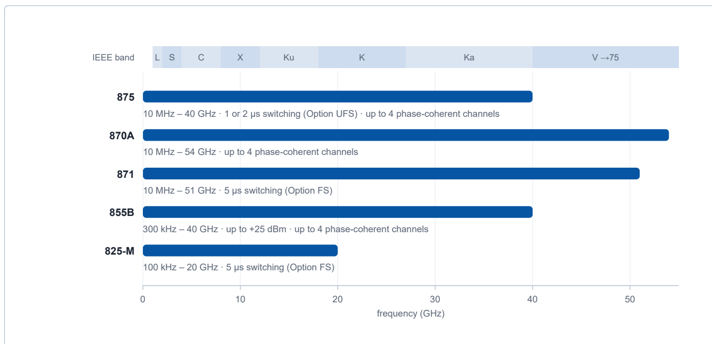
■ DERIVED Figure 1. Frequency coverage of the recommended sources against the IEEE radar bands, top-of-family versions, from the current datasheets.
