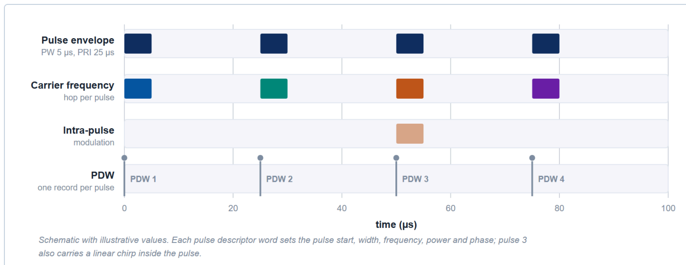
■ SCHEMATIC Figure 2. A frequency-agile pulse train, one PDW per pulse setting start, width, frequency, power and phase, with an intra-pulse chirp on the third pulse; illustrative values.
