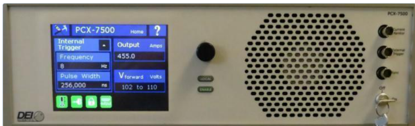
■ PHOTO Figure 3. PCX-7500-EX pulsed current source, front panel, with the trigger, pulse-width and output settings on the touchscreen.
