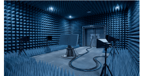
Illustration: an anechoic chamber with a receive array on a positioner and four horn antennas on stands around it.
