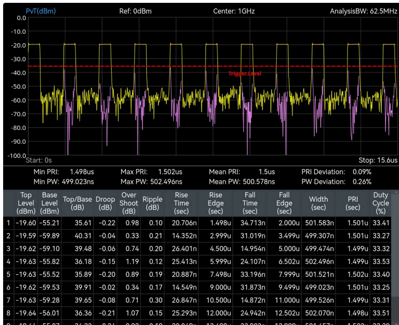
MEASURED Figure 3. Pulse Detection (option 72) on a 1 GHz pulse train, 62.5 MHz analysis bandwidth, reference level 0 dBm, 15.6 microsecond record. Mean PRI 1.5 microseconds, mean pulse width 500.6 ns, duty cycle 33 percent; the table lists level, rise and fall time, width, PRI and duty cycle for every pulse.
