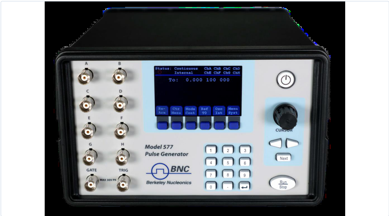
Figure 3. The Model 577 benchtop: eight output connectors, A through H, down the left of the panel with the gate and trigger inputs below them, a color display with soft keys, keypad and cursor knob. The display's status line lists all eight channels at once, and the panel itself marks the input pair at 30 V peak maximum, the conservative limit this handbook quotes. PHOTOGRAPH
