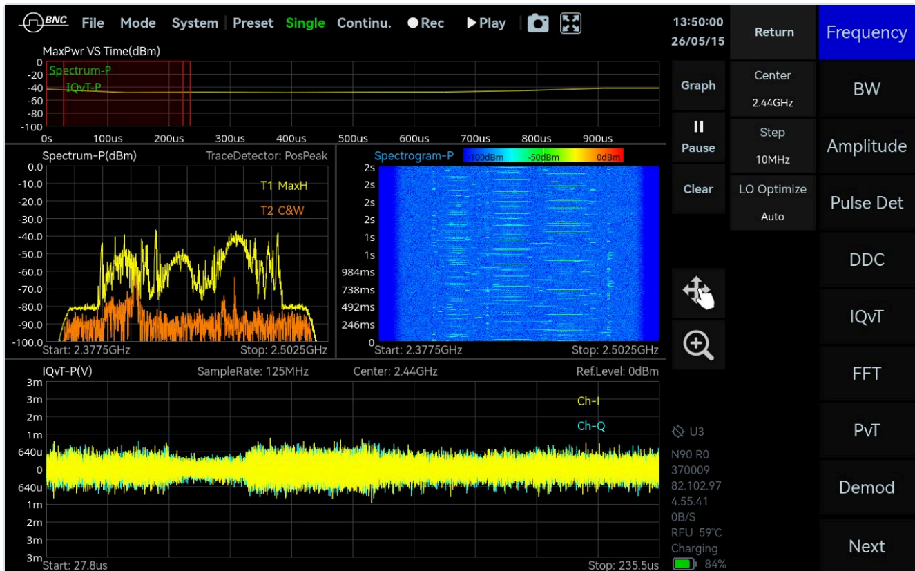
Figure 16. One acquisition presented four ways at once: power against time, max-hold and clear-write spectra, a two-second spectrogram, and I and Q across a 208 microsecond window with a sample-rate field reading 125 MHz. The span reads 2.3775 to 2.5025 GHz, which is 125 MHz: the sample rate rather than the usable 100 MHz , which is the confusion section 16 warns about, visible here as a setting. Read the spectrogram against the buffer arithmetic rather than past it: two seconds is far longer than the buffer holds at this rate, so that pane is a live rolling display and the IQ pane below it is the buffered case. MEASURED
