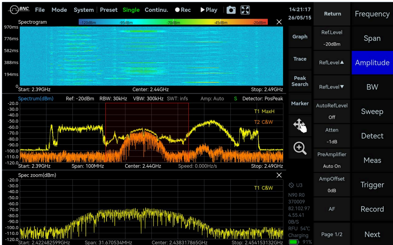
Figure 8. The 2.4 GHz band held whole: 2.39 to 2.49 GHz in one 100 MHz window at 30 kHz resolution, with max hold and a single sweep overlaid in the center pane, a spectrogram above and a 31.67 MHz zoom below. Read the gap between the two traces. The upper trace is what accumulation finds; the lower one is one instant. Where they differ, by 20 dB and more in places, is exactly what a receiver that visits this band rather than holding it would have reported as empty, and the difference is a function of when it happened to look rather than of what was there. MEASURED
