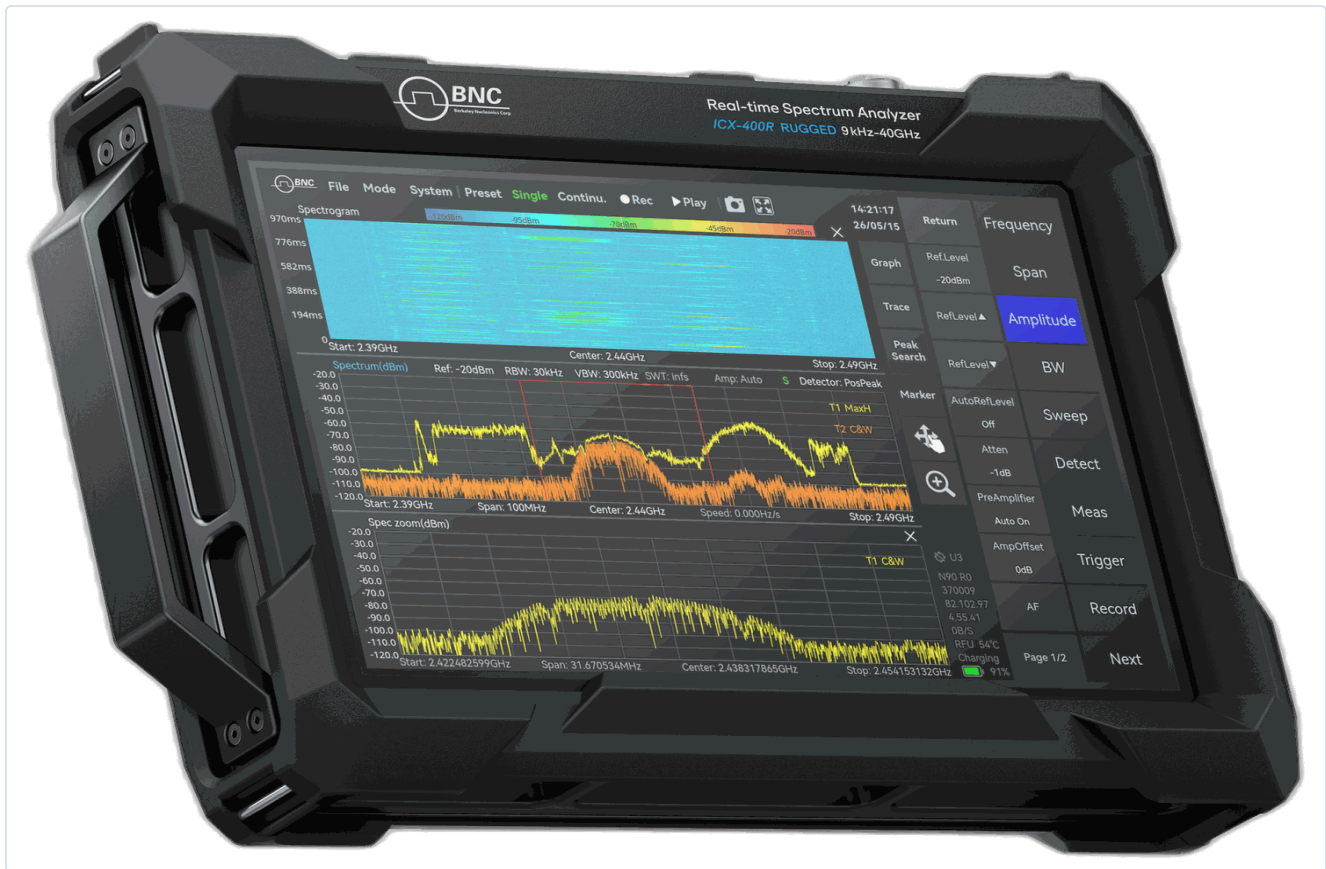
Figure 17. A product render of the rugged tablet, not a photograph, and the screen it carries is the capture already shown as Figure 8 rather than a second measurement: the timestamp, the spans, the temperature and the battery state all match it exactly. It is here to show the form factor, and the bezel reading ICX-400R, 9 kHz to 40 GHz, is the only thing in the image offered as evidence of anything. The published interface list is identical across all three form factors, the same languages, the same SCPI and the same measurement set, which is what makes a routine written against a module on a bench portable to this one. That the datasheets agree is published; that any given routine moves untouched follows from it as a reasonable inference, and is worth confirming for your own routine before you plan around it. It is the practical content of buying a line rather than a product. SCHEMATIC
