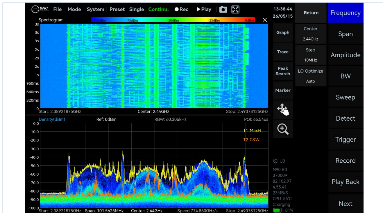
Figure 5. The engine on the glass: real-time density with its spectrogram, 2.389 to 2.491 GHz in a 101.56 MHz span at 60.3 kHz resolution, with the display reporting a 65.54 microsecond probability of intercept. That figure is 2 \times 4096 \times 8 ns to the four digits the display carries, so the relation of equation (2) is visible here as a reading at a transform size no datasheet quotes. The span field reads 101.56 MHz, above the published 100 MHz analysis bandwidth, for the same reason the sample-rate field exceeds it elsewhere: the number is the transform's extent rather than a claim about usable bandwidth. Density accumulates every transform rather than the peak of a sweep, so an intermittent emitter resolves into a persistent trace with its duty cycle visible instead of an occasional spike.
