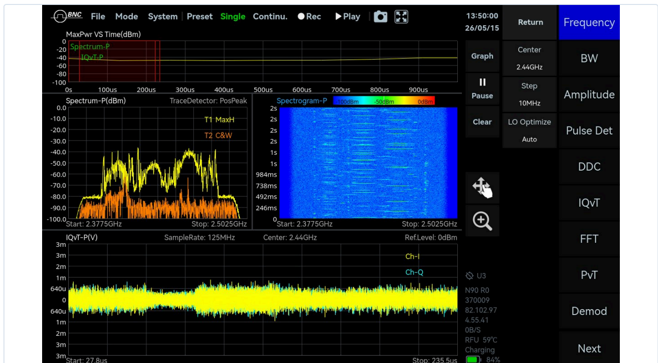
Figure 6. One acquisition presented four ways at once: power against time, max-hold and clear-write spectra, a two-second spectrogram, and I and Q across a 208 microsecond window with a sample-rate field reading 125 MHz. The span reads 2.3775 to 2.5025 GHz, which is 125 MHz, the sample rate rather than the usable 100 MHz, and that gap is the convention section 6 warns about visible as a setting. Read the spectrogram pane against the buffer arithmetic rather than past it: it covers two seconds, far longer than the 0.26 s the buffer holds at this rate, so the spectrogram is a live rolling display and not a view of one buffered acquisition. The IQ pane below it is the burst case of the table above. MEASURED
