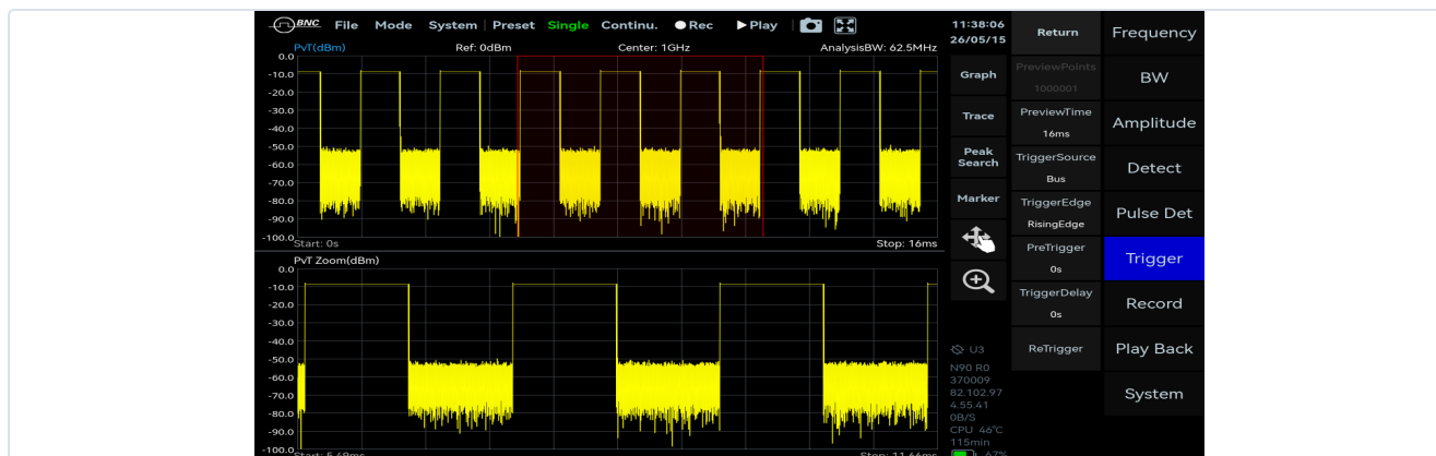
Figure 4. Power against time turns duty cycle from a declared parameter into a measured one: a pulse train at 1 GHz in a 62.5 MHz analysis bandwidth over a 16 ms record. The pulses drawn here are milliseconds apart rather than the microseconds of a 5G burst set, so read it for the method rather than for its numbers. Assuming a higher duty than the frame runs over-states the maximum, which is safe. It is the reverse that hurts: a frame declared at 0.55 but actually running at 0.743 costs 1.3 dB in the non-conservative direction.
