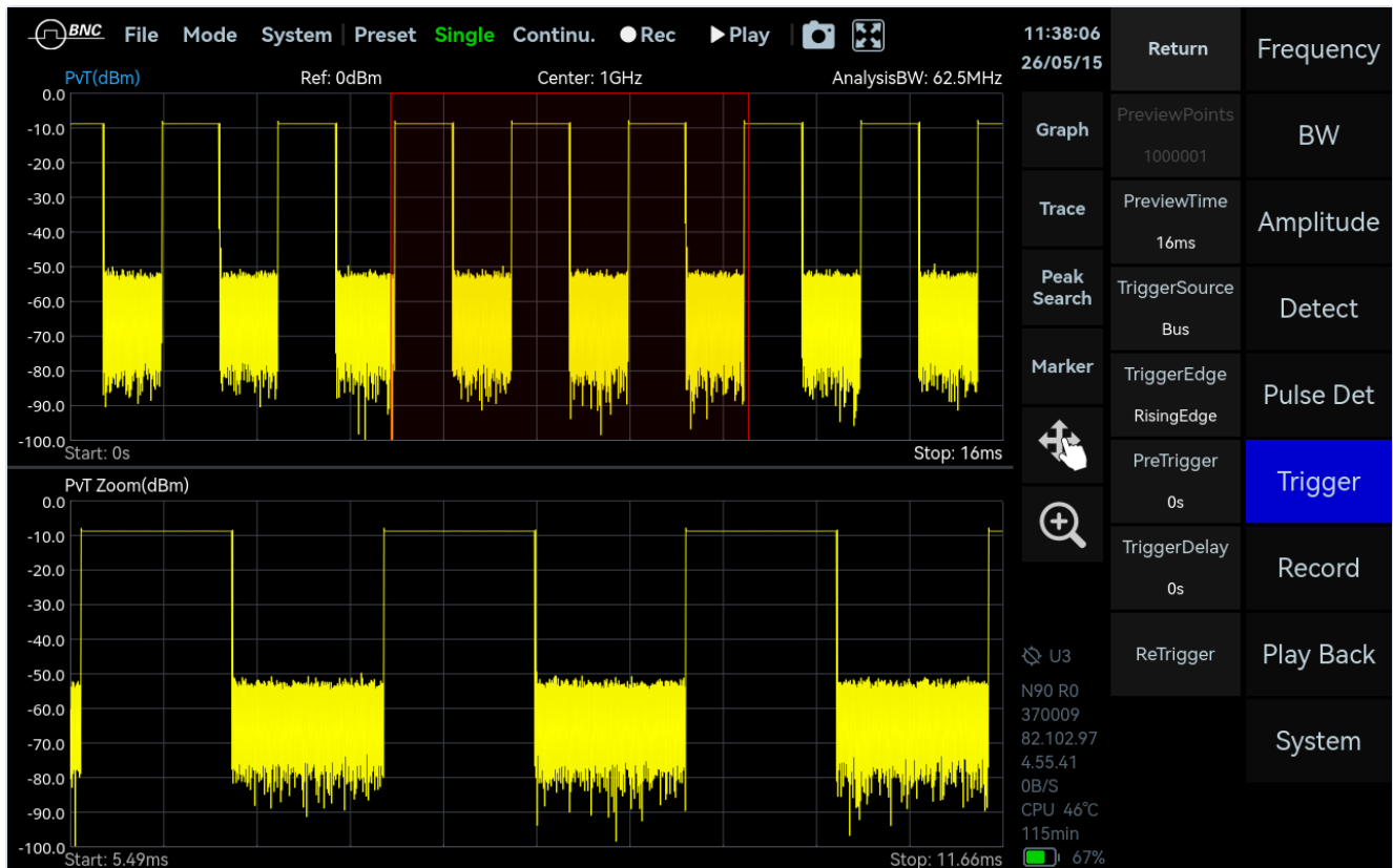
Figure 4. Power against time is the measurement that produces a pattern point: a pulse train at 1 GHz in a 62.5 MHz analysis bandwidth, a 16 ms record with a zoom on 6 ms of it, tops flat at -10 dBm and bases at -50. The pulses here are milliseconds apart rather than the microseconds of the worked case, so read it for the shape of the measurement rather than for its numbers. One cell yields hundreds of pulse amplitudes, and the statistic of that population is what carries an honest null depth. MEASURED
