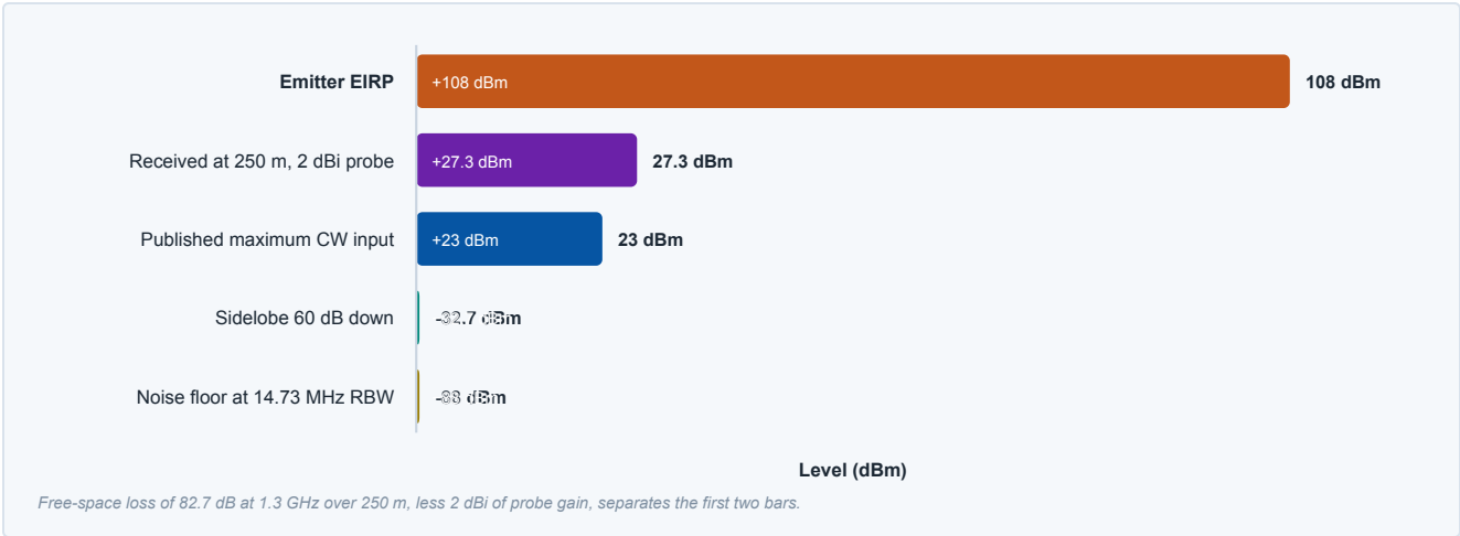
Figure 6. The dynamic-range problem on this flight is at the top of the scale, not the bottom. The received main beam sits 4.3 dB above the published input maximum while the sidelobe of interest sits 55 dB above the noise floor, so a pad costs nothing that matters and its absence costs the measurement. DERIVED
