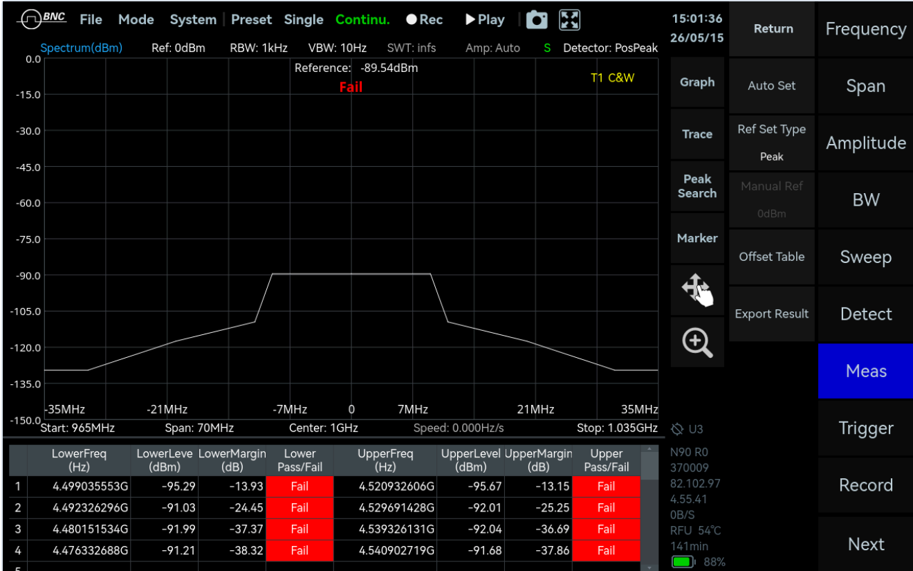
Figure 6. The spectral emission mask function in SpectraCore: a stored mask template over a 70 MHz span at 1 kHz resolution bandwidth, 10 Hz video bandwidth and peak detector. This is a bench illustration of the function, not a Ku-band earth-station capture. Shoulder levels against the operator's mask are the compliance record a regrowth accusation is answered with, and they are worth capturing at more than one back-off setting so the trade is documented rather than argued. MEASURED
