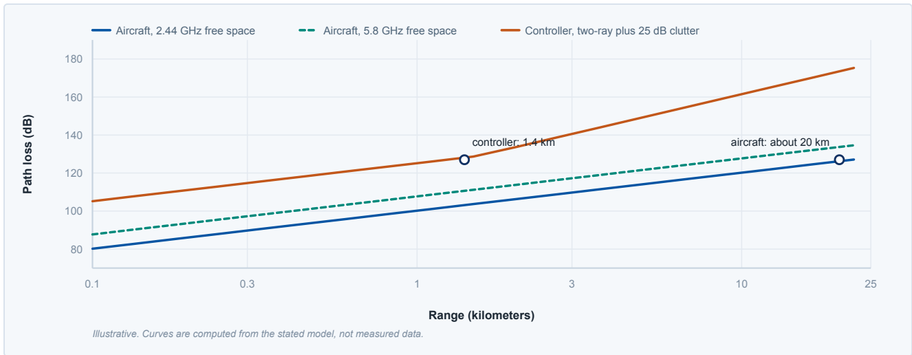
Figure 4. At identical transmit power the aircraft is detectable roughly fourteen times further than its controller. The difference is not power. It is ground reflection and clutter standing between the sensor and the person you are trying to find. DERIVED
