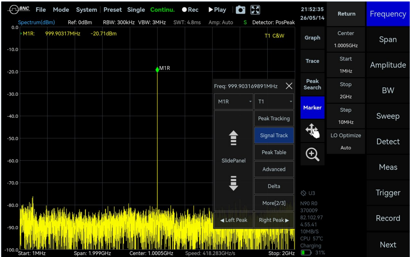
Figure 5. Marker signal track holding a drifting carrier at 999.90 MHz in SpectraCore: 1 MHz to 2 GHz span, 300 kHz resolution bandwidth, peak detector. This is the limit of what one channel can prove about one emitter. A bearing needs the same burst on several channels at once, and no single-channel display can show that. MEASURED
