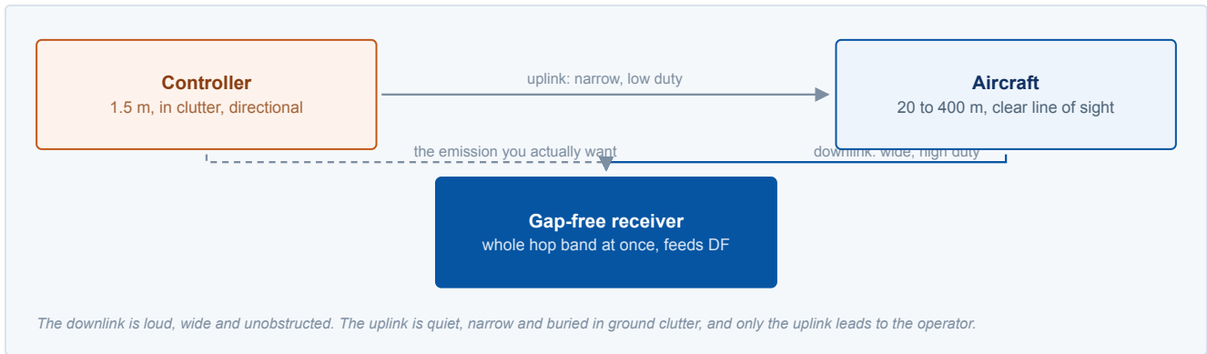
Figure 1. Two emitters, two geometries, two problems. Detection is usually won on the downlink and the operator is only ever found on the uplink, which is the harder of the two by twenty to forty decibels of geometry alone. SCHEMATIC
