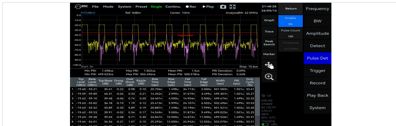
Figure 6. The parameterization stage doing its job: 500 ns pulses at a 1.5 microsecond interval, centered at 1 GHz in a 62.5 MHz analysis bandwidth, with a per-pulse table of level, droop, overshoot, ripple, rise and fall times, width, interval and duty cycle. The displayed 15.6 microsecond record holds about ten pulses and the analyzer accumulates the requested hundred into the table, where the measured interval deviation of 0.09 percent is the kind of feature a classifier keys on. It exists because pulse detection measures in the time domain with a dedicated detector rather than through the transform path, so the intercept boundary of section 3 does not apply to it; what the gap-free front end guarantees is that no pulse in the record is missing. MEASURED
