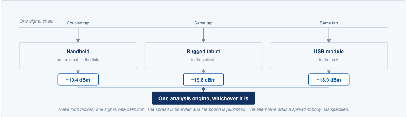
Figure 2. The same tap measured by three form factors under one analysis engine. The three readings differ, and they are allowed to: all three are within one stated amplitude bound and they are the same quantity, so the spread is known. Assemble the fleet from three vendors and the readings differ by that bound plus each vendor's reference conventions, which is a difference no calibration certificate removes because every one of the three is individually correct. SCHEMATIC
