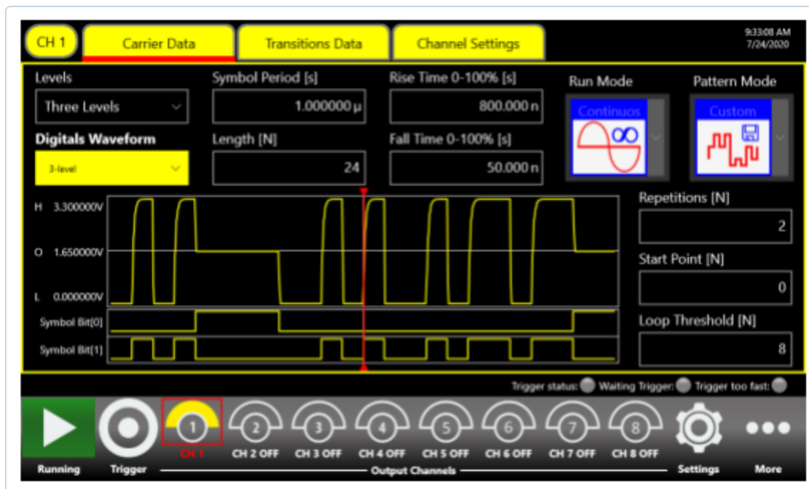
■ MEASURED Figure 1. Carrier data page of the control software with a three-level custom pattern: levels 0, 1.65 and 3.3 V, symbol period 1 μs, 24 symbols, rise time 800 ns, fall time 50 ns.
