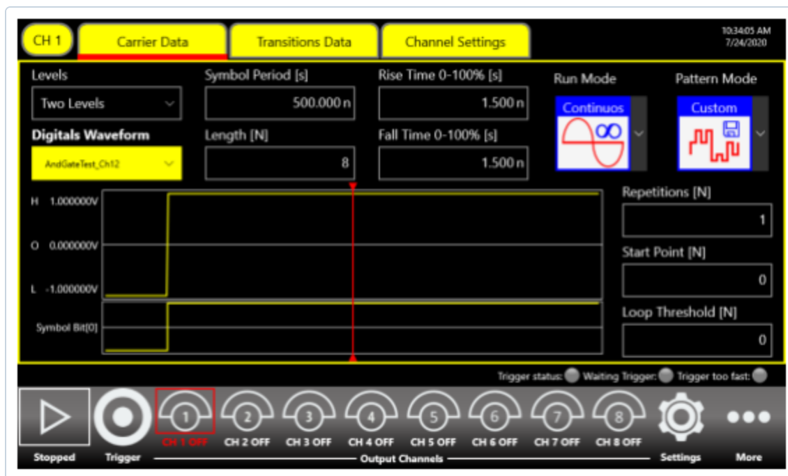
MEASURED Figure 7. Carrier data page for the propagation-delay test: two levels, symbol period 500 ns, 8 symbols, rise and fall 1.5 ns.
