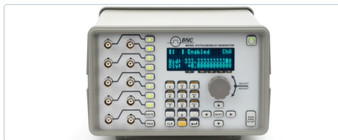
PHOTO Figure 4. Model 575 Digital Delay/Pulse Generator: 250 ps delay and width resolution per channel; 50 ps RMS internal rate generator jitter and 800 ps RMS external trigger jitter; individual rates per channel; dual inputs, gate plus trigger or two triggers with Option DT15; USB and RS-232 standard, Ethernet and GPIB with Option COM.
