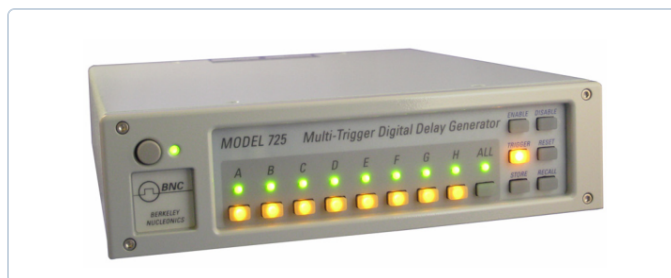
PHOTO Figure 5. Model 725 Multi-Trigger Digital Delay Generator: trigger-pulse delay 20 ns to 1370 s; eight external inputs and eight outputs, with seven internal logic inputs feeding the eight timing processors; delay jitter from an internal source 50 ps typical, 200 ps maximum; external trigger pulse 50 ns minimum.
