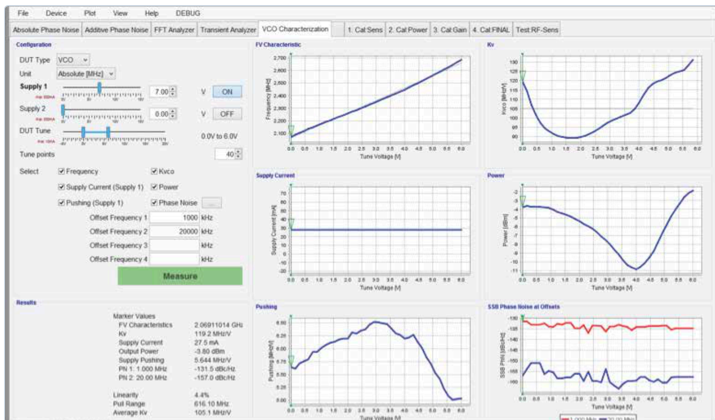
MEASURED Figure 5. GUI screen of a completed VCO characterization over 40 tuning points from 0 to 6 V, showing frequency, tuning sensitivity, supply current, output power, supply pushing and SSB phase noise at 1 MHz and 20 MHz offsets.
