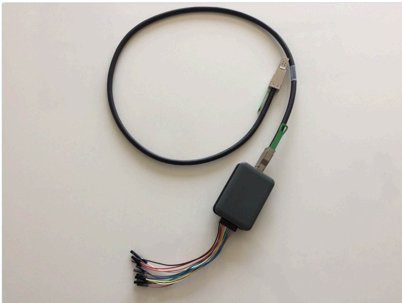
■ PHOTO Figure 2. The AT-DTLL8 probe on its one meter mini-SAS HD cable, with the single-ended output leads.
