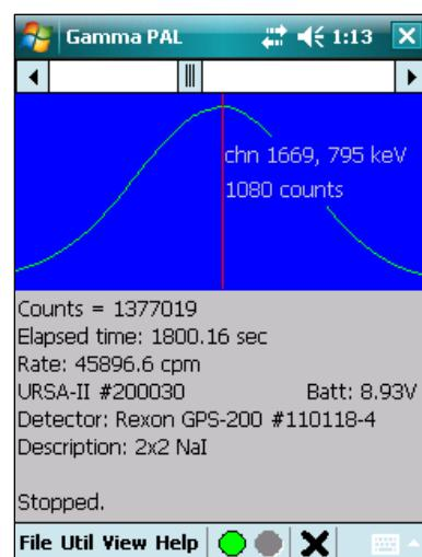
manufacturer, model, serial number, and the detector description. The final line contains relevant information on acquisition status, background status, etc.
