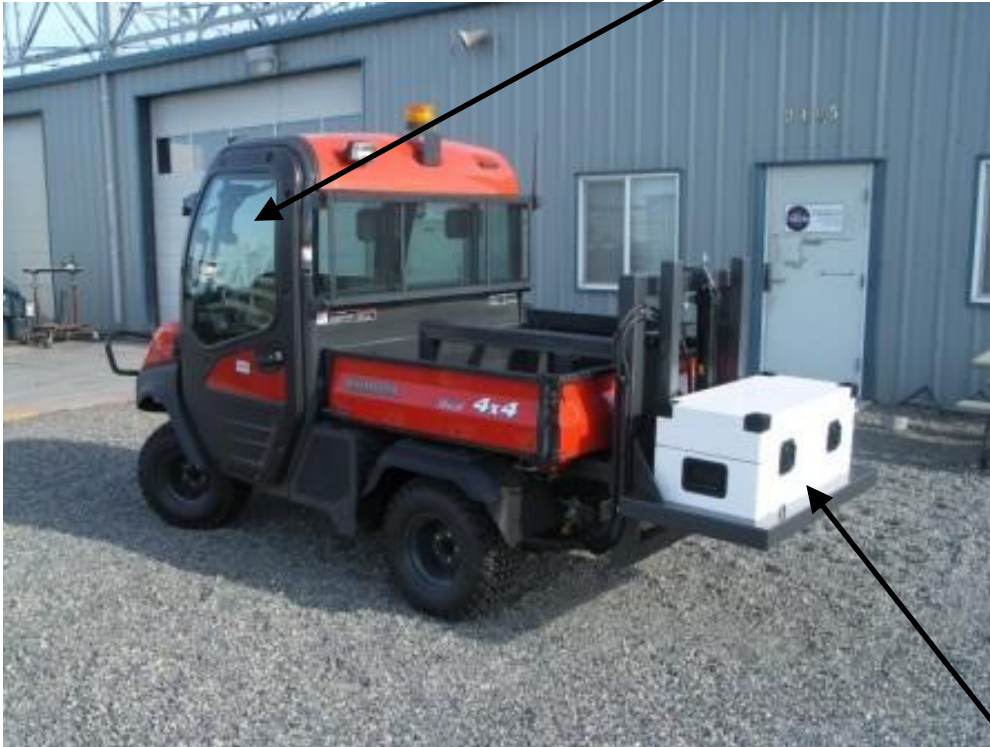
Large Volume NaI Detector in Shock Absorption Package
