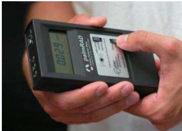
An electronic dosimeter detects and computes radiation and the amount of exposure. Berkeley Nucleonics officials say there is no need for homeowners to worry that their kitchens emit radon. (IJ photo/Alan Dep)
