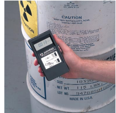
palmRAD 904 shown above. Used to locate radiation and measure in uR.
